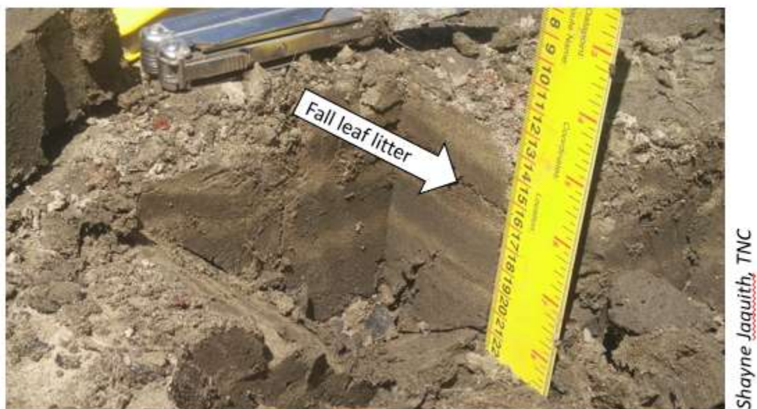
Figure 1. Identify contact between fresh sediment deposit and underlying organic layer.
