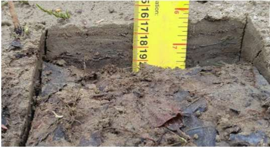
Figure 2. Fresh sediments removed from a 15 cm x 15 cm square down to the underlying organic layer (i.e., leaf litter from previous fall).
