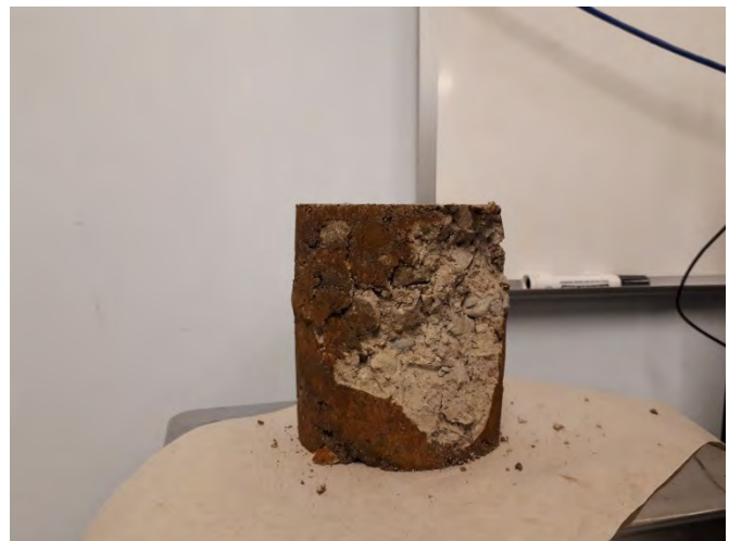
Figure 3.17. The dried, tested 6% LLC 28 days oven cured specimen.
