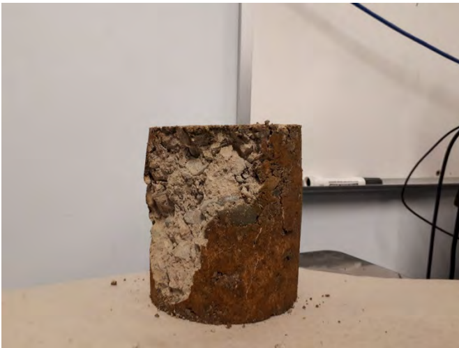
Figure 3.17. The dried, tested 6% LLC 28 days oven cured specimen.
