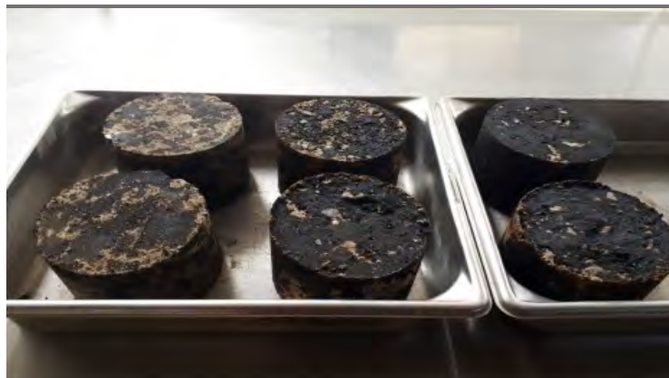
Figure 2.16. Photo of the prepared asphalt emulsion specimens
