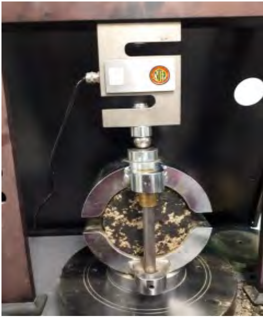
Figure 2.17. Testing of the prepared asphalt emulsion specimens
