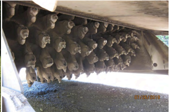
(b) Teeth on grinding/mixing drum of Wirth 2500S reclaimer used on the project.
