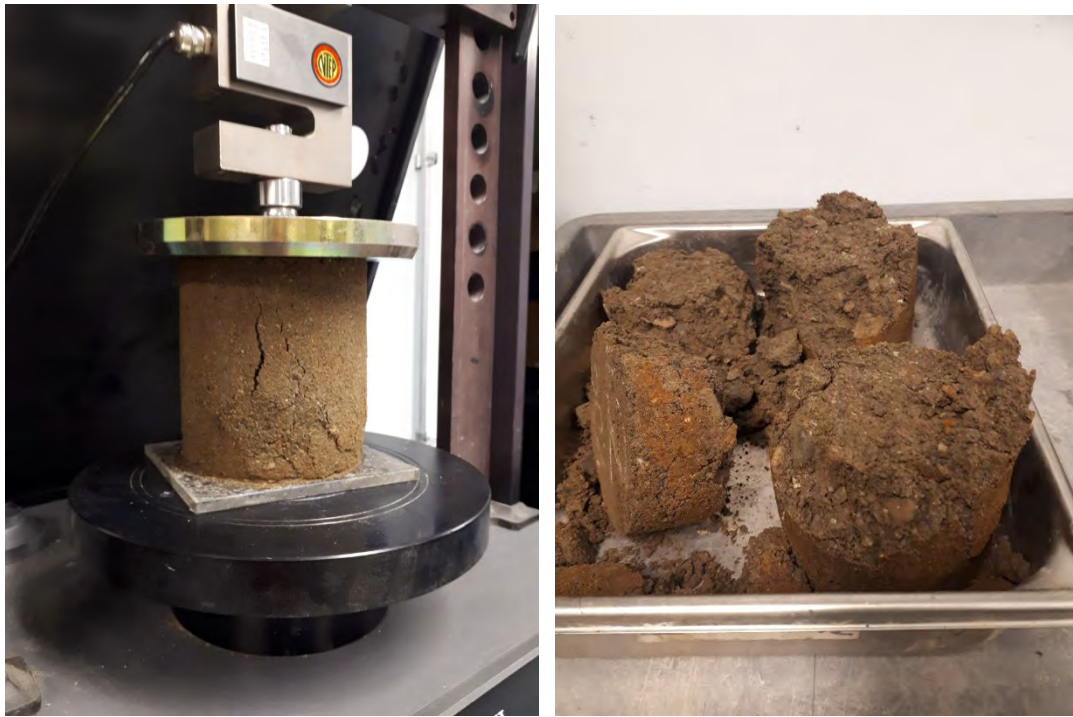
Figure 3.21. Moist specimens of Subbase III after the end of the curing period
