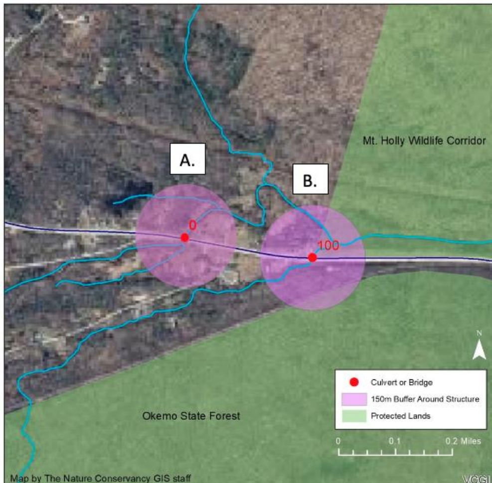
Figure 5. Protected lands analysis around two structures on VT Rt. 103 in Mt. Holly, VT. Structure A has no adjacent protected land blocks and receives a score of 0 based on the analysis criteria. Structure B receives a score of 100 due to the presence of two large blocks of protected land occurring on both sides of the roadway and within the buffered analysis area around the structure.
