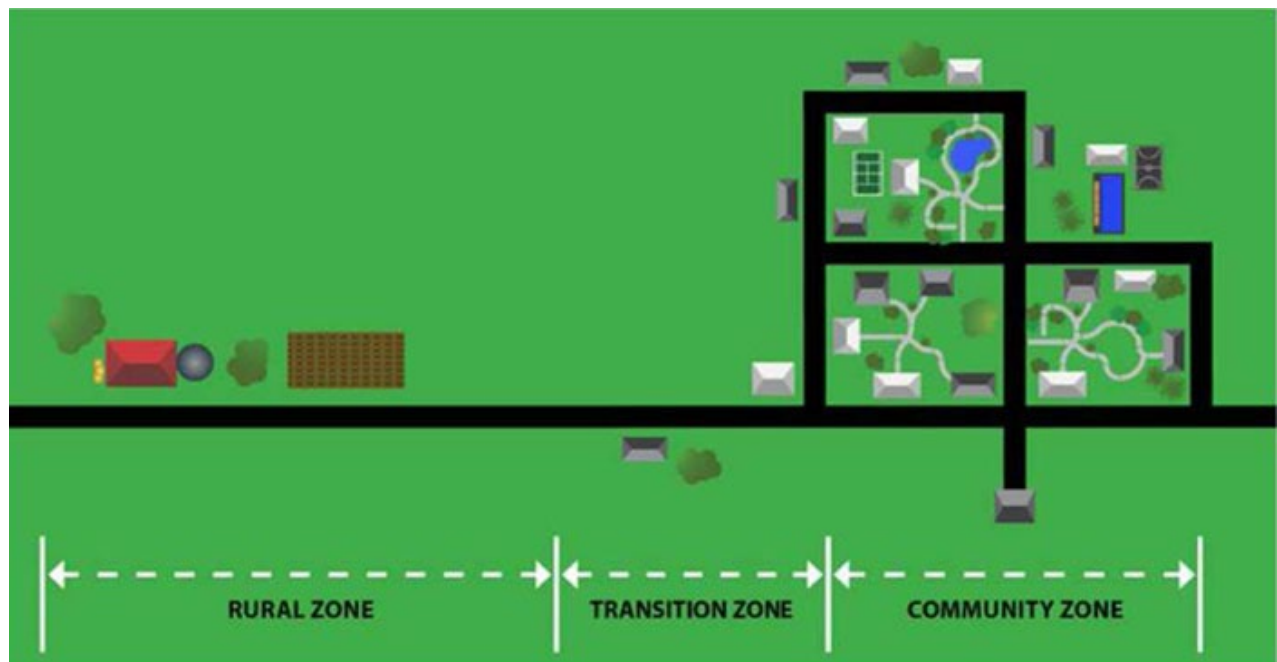
Diagram of a rural highway transition zone into a village or town center (FHWA, 2018)
