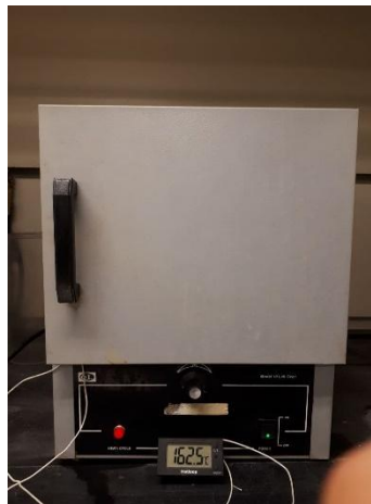
Figure 16 - Photo of the portable oven used to heat the HMA mixture components.
