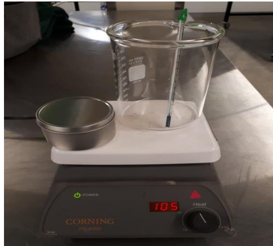
Figure 17 - Boiling water test setting
