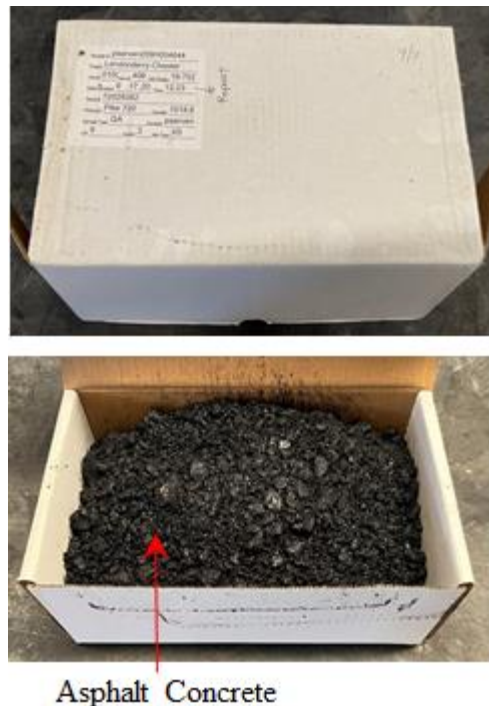
Figure 11 - Plant Produced HMA mixture from Londonderry-Chester Project
