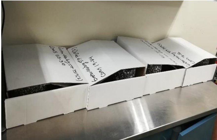
Figure 14- Storage of the boxes with asphalt cores on a flat surface
