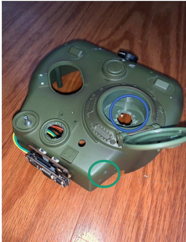
Figure 86 Holes drilled for antenna
