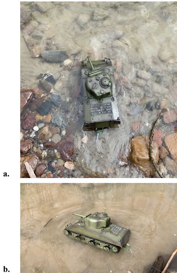
Figure 11 Waterproofed HIVE 2.0 tested for water tolerance in a stream
