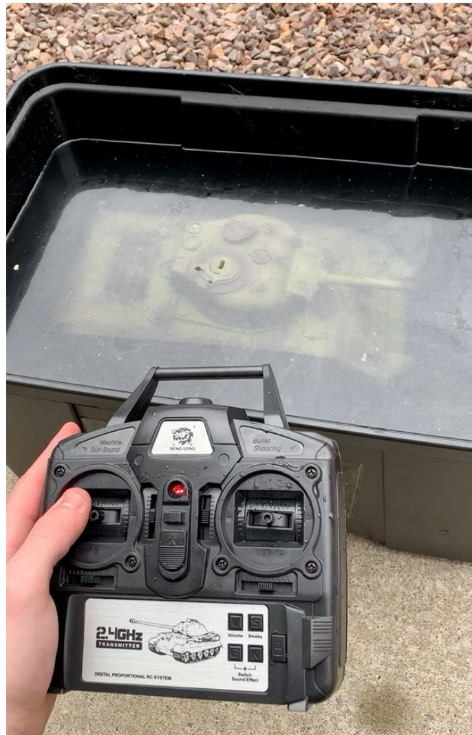
Figure 10 Submersion test of HIVE 2.0 tank that successfully operated under water with wireless remote-control telemetry
