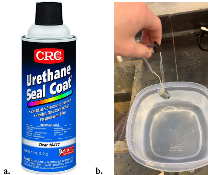
Figure 9 Waterproof coating submersion test: a. Polyurethane spray coating, and b. Submersion test of coated running DC electric motor
