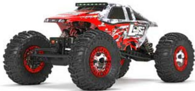
Figure 4 Losi Night Crawler 2.0 with 4-wheel drive and worm-gear differentials that provide self-braking [Losi 2020]
