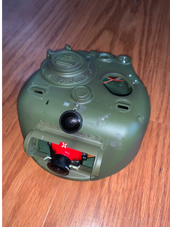
Figure 83 Camera 2 position in turret
