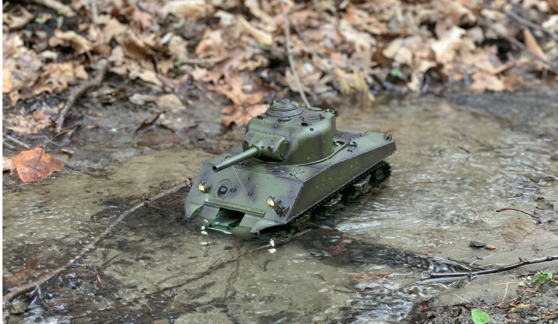
Figure 15 Stream testing confirms viability of cutouts and holes in reducing lift and drag of flowing water on HIVE 2.0 tank
