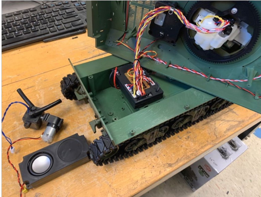
Figure 70 Tank with speaker and smoke generator removed
