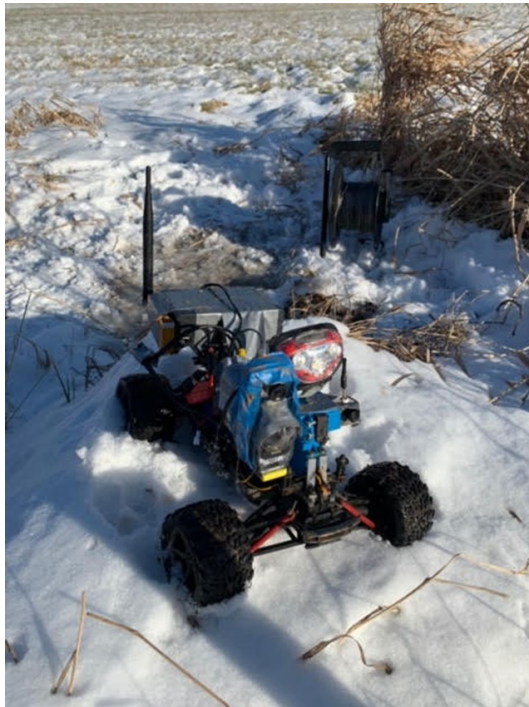
Figure 37 Telemetry Option Test 1 using HIVE 1.0 instrumented with 1.2, 2.4, and 5.8 GHz video systems: a. HIVE 1.0 with added telemetry options, and b. Setup with telemetry modules and retrieval wire spool
