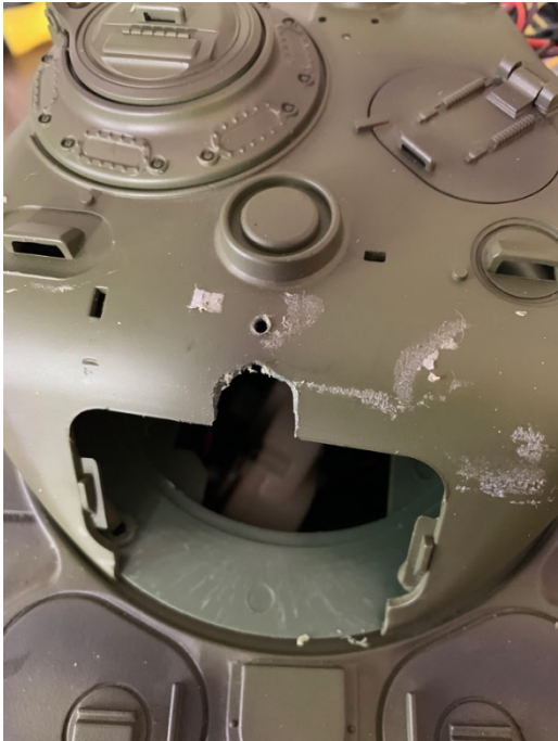
Figure 76 1/2-inch hole drilled for Camera 1 mounting
