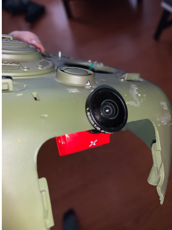
Figure 78 Camera 1 position in turret
