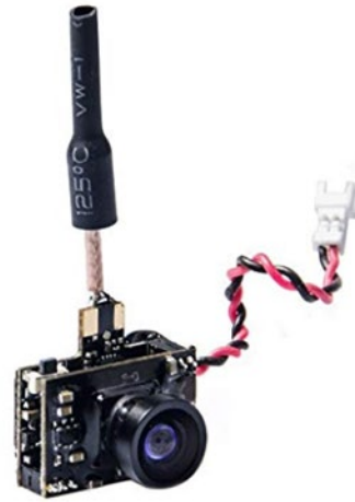
Figure 35. Camera with integrated 5.8 GHz transmitter
