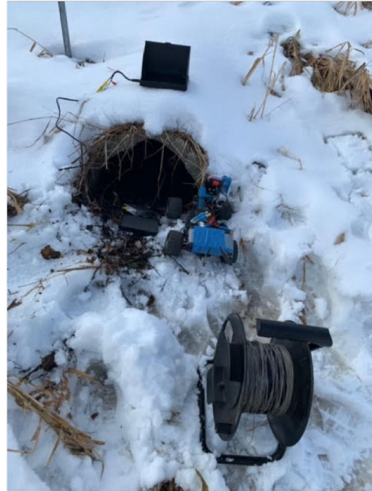
Figure 37 Telemetry Option Test 1 using HIVE 1.0 instrumented with 1.2, 2.4, and 5.8 GHz video systems: a. HIVE 1.0 with added telemetry options, and b. Setup with telemetry modules and retrieval wire spool
