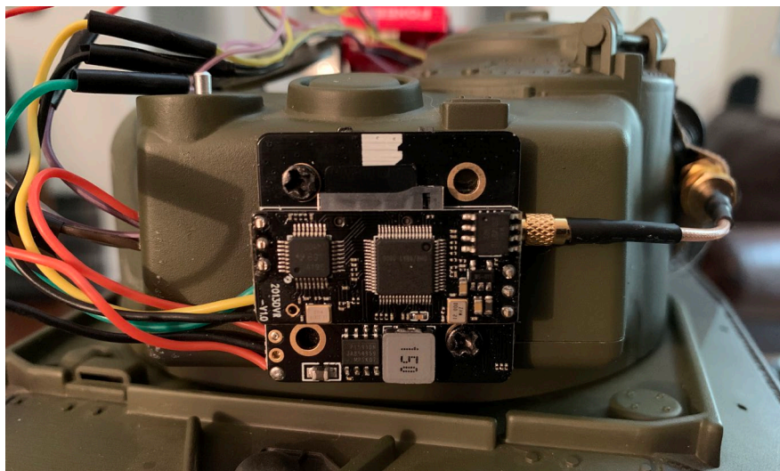
Figure 85 Transmitter board attached to back side of turret in assembled HIVE 2.0 tank
