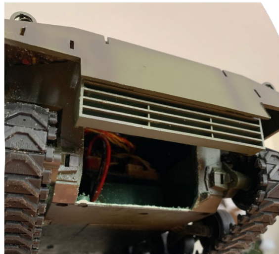
Figure 14 Cutouts in HIVE 2.0 tank body to allow free flow of water: a. Front with cutout, and b. Back with cutout
