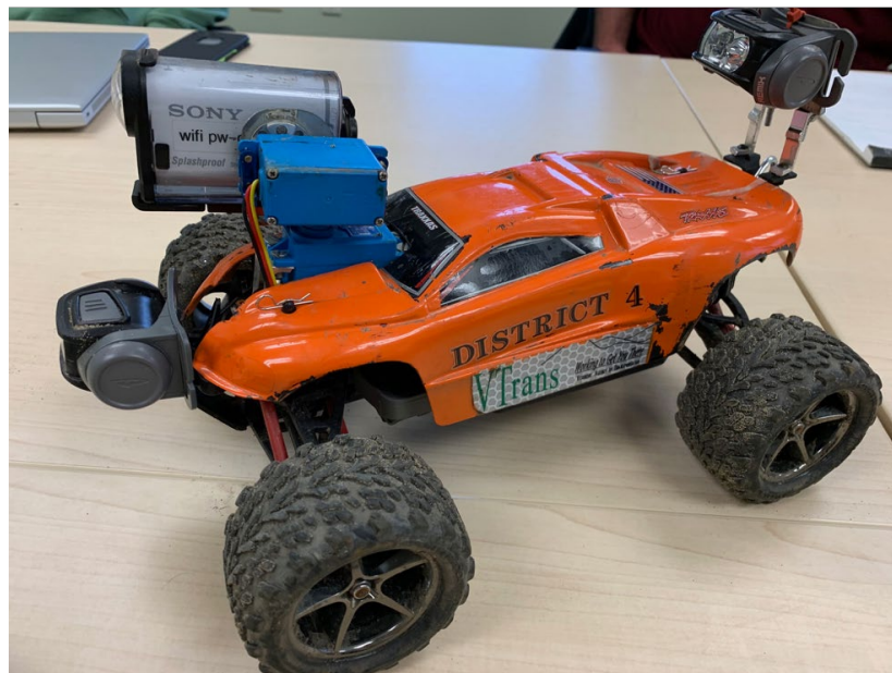
Figure 2 HIVE 1.0 used by VTrans with articulated Sony Action Cam video camera mounted on two servo motors
