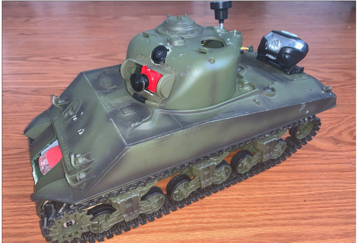
Figure 18 Modified HIVE 2.0 showing water passage cutout in front, modified turret with forward looking and elevated cameras, jogging headlamp light and circular antenna.
