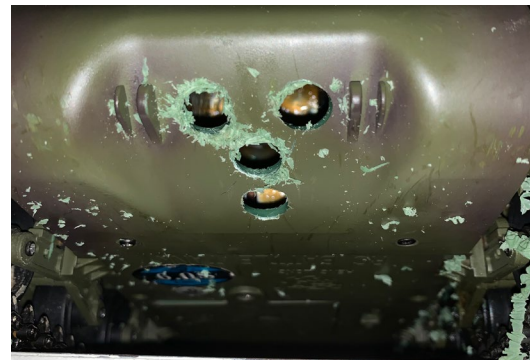
Figure 13 Holes drilled into HIVE 2.0 tank to allow internal flow of water and reduce drag: a. Side undercarriage, b. Bottom
