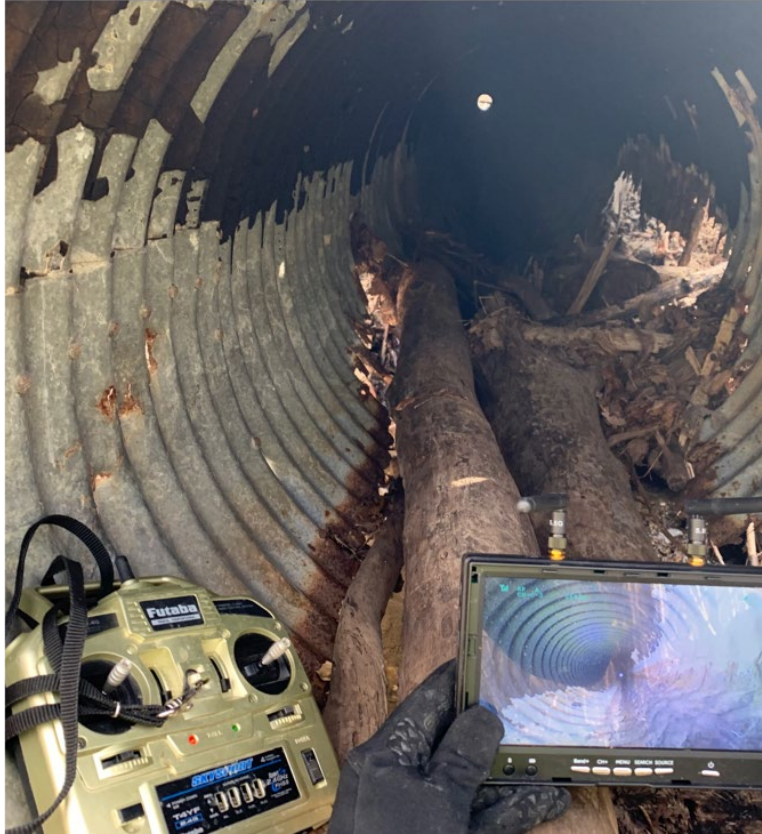
Figure 42 Test 2 setup, monitor at exit of Culvert 64099 with vehicle at entrance
