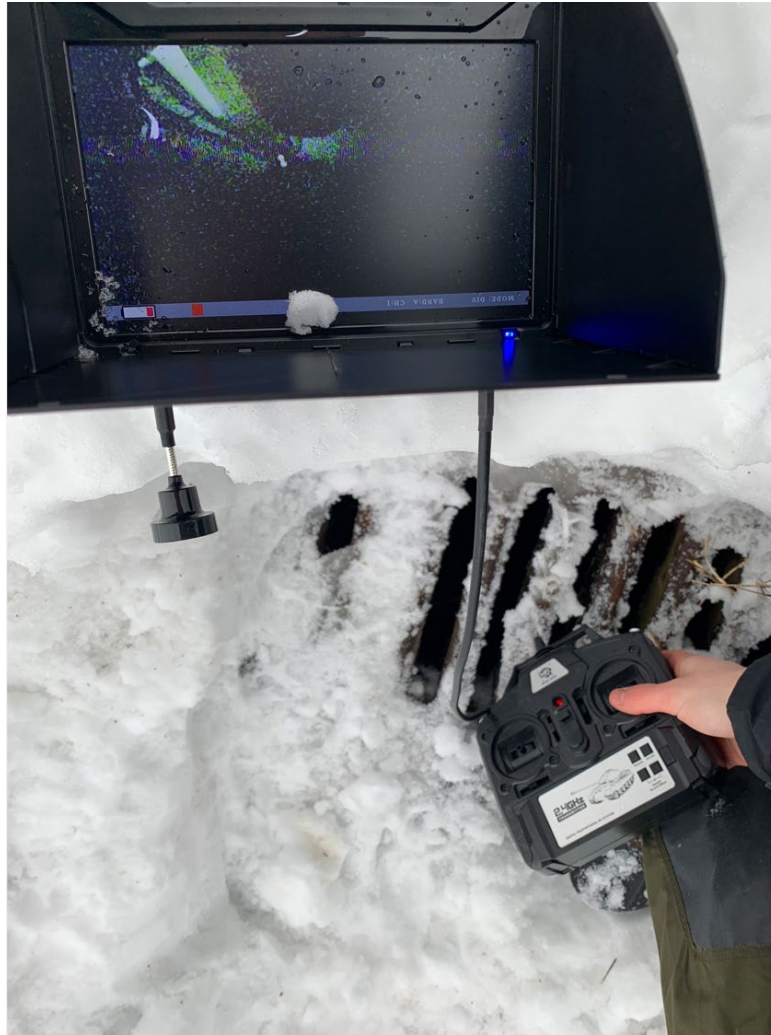
Figure 55 Tank remote held above middle DI grate to drive HIVE 2.0 tank back to exit
