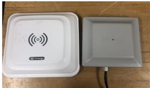
Fig. 11. The two antennas acquired: Invengo (left) and SecureControl (right)
