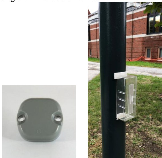
Fig.23. Tag mounting of Omni-ID Exo 750 (left) and Omni-ID Flex 1200 (right).
