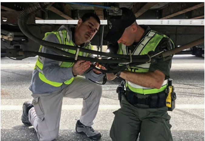
STATEWIDE. DMV's certified inspectors conduct a Level I Inspection, a 37-step procedure that includes an examination of driver operating requirements and vehicle mechanical fitness.
