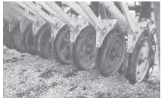
Depth control bands ensure uniform, shallow seed placement.
