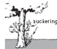
Figure 13. Suckering is one symptom of construction damage.
