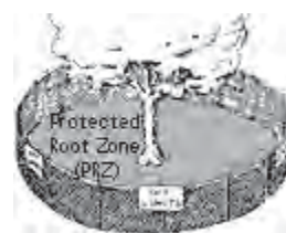
Figure 5. Put up fences and signs around trees you want to save to alert construction workers to damage potential.
