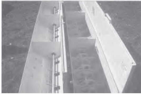
Seed box agitators help to maintain an even flow of native grass seeds to the furrow openers.
