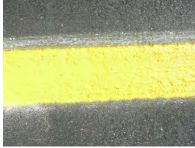
Figure 3: Close-Up View of Glomarc 90 Spray-Applied with VISIBEAD™
