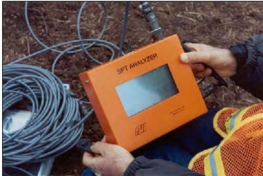
Figure 12 Photograph of the SPT Analyzer Data Acquisition Box.
