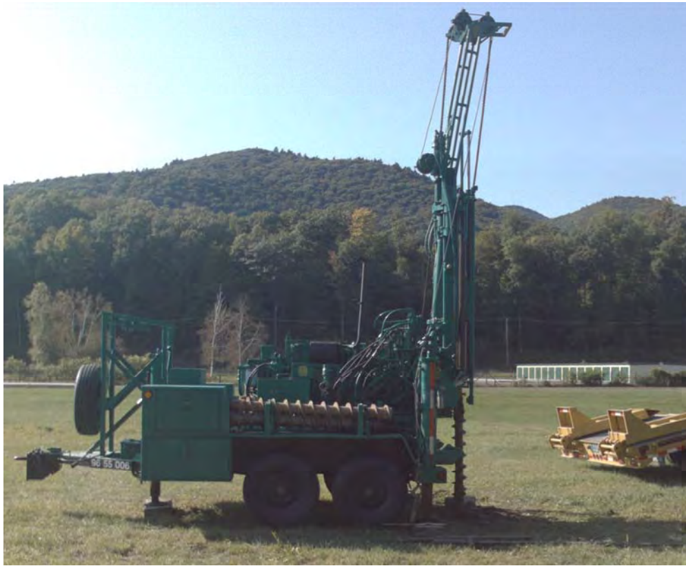
Figure 2 VTrans CME 45C Skid Rig on Trailer used on Boreholes GD-2 and GD-4.
