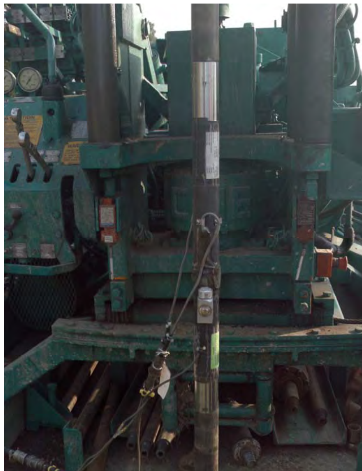
Figure 10 AWJ instrumented Drill Rod.
