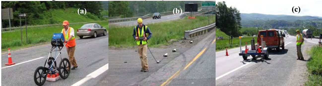
Figure 6.1 (a) GSSI cart-mounted GPR. (b) Geometrics OhmMapper CCR towed array. (c) Dynatest® FWD trailer system.
