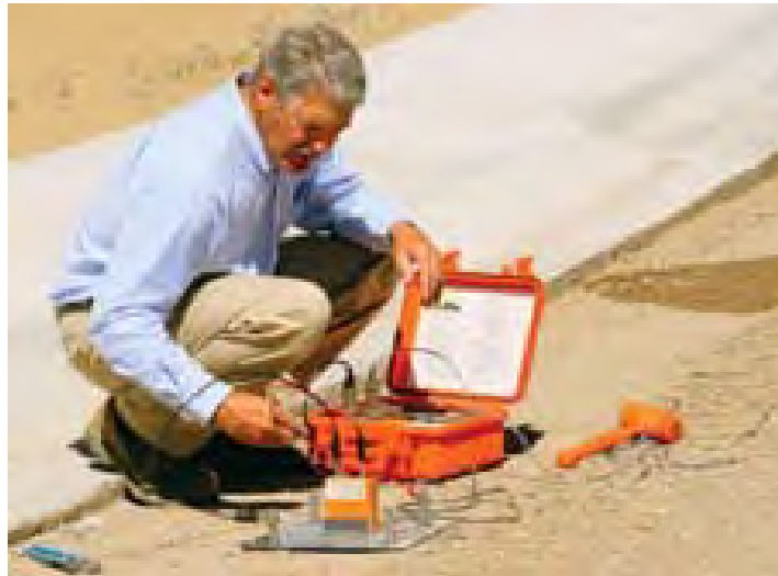
Figure 4: Typical EDG test set-up
