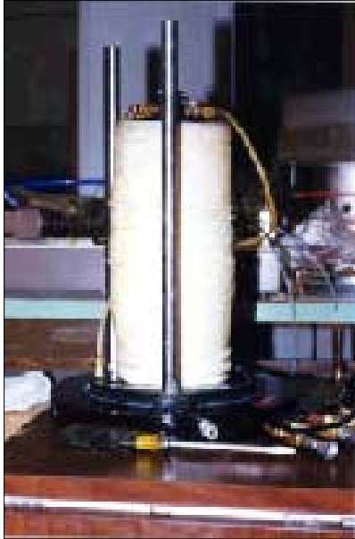
Figure 16. 150-mm-diameter test specimen at the end of testing.
