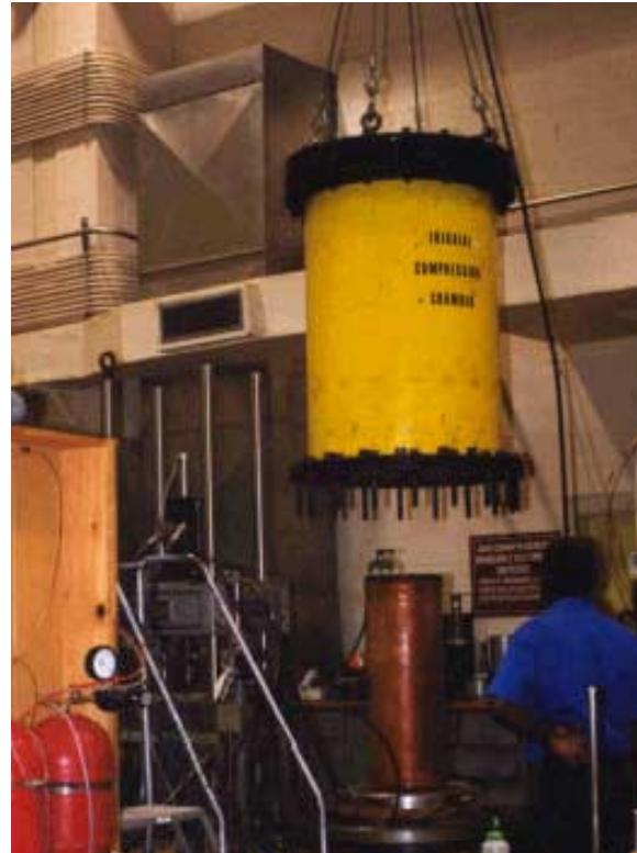
Figure 11. Placement of triaxial chamber around test specimen.
