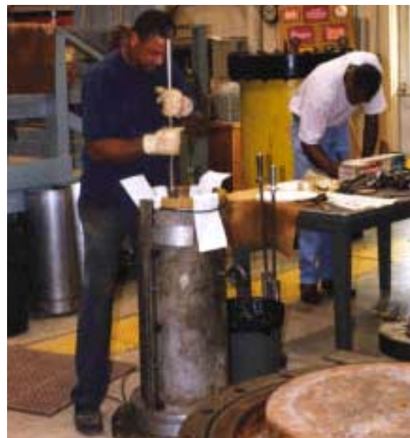
Figure 9. Specimen preparation for resilient modulus test.
