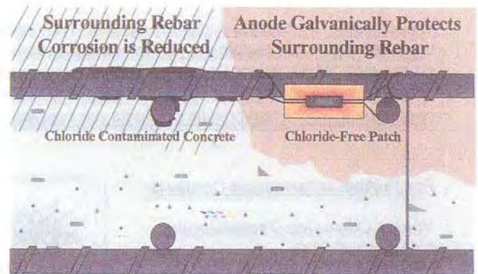
Galvashield XP Reduces "Ring Anode" Corrosion
