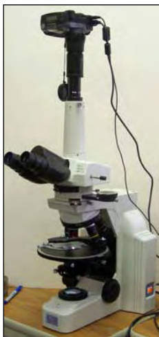
Figure 2 Petrographic Microscope (notice Kodak DC-290 Digital camera mounted on phototube).
