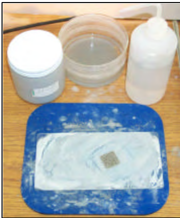
Figure 9 Photograph showing hand lapping equipment.
