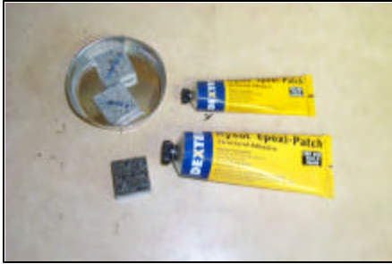
Figure 2 Mortar bar cubes and two-part epoxy used to bind sample to slide .
