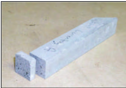
Figure 1 Mortar bar showing \frac{3}{4} " cube cut from bar. Cubes were cut utilizing a Raytech 10" Trim Saw cooled with RV propylene glycol antifreeze coolant.
