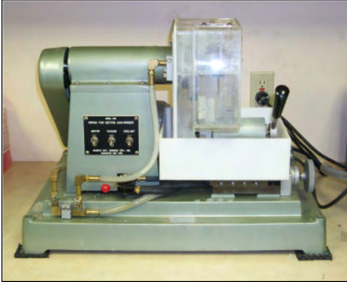
Figure 8 Thin section saw/grinder used to prepare sample. This equipment allows the sample to be ground down to 30 microns or less.
