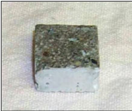
Figure 3 Mortar bar cube showing epoxy coated surface.
