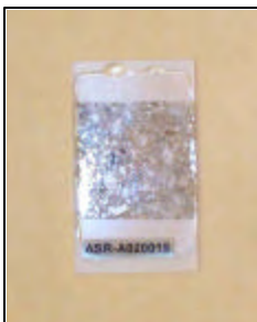
Figure 10 Completed thin section slide. This slide contains a sample that is 30 microns in thickness. This allows the sample to be analyzed using the petrographic microscope.
