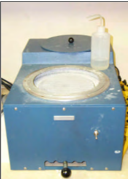
Figure 4 Grinder/Polisher used to prepare sample for mounting to slide. Samples were polished by holding the cube to the wheel using progressively finer grit disks while carefully applying water to cool the sample and to wash away waste cuttings.
