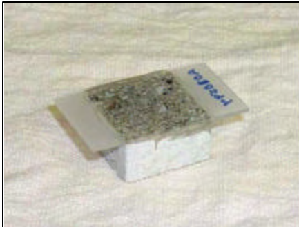
Figure 6 View of underside of epoxied sample.
