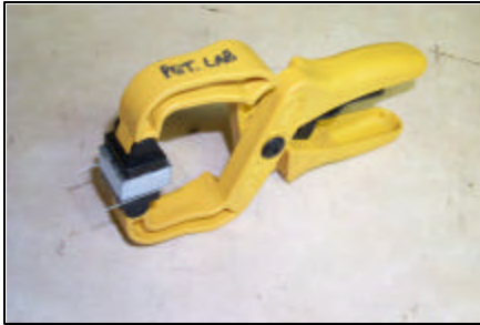
Figure 5 Clamp used to hold slide securely to sample while curing.
