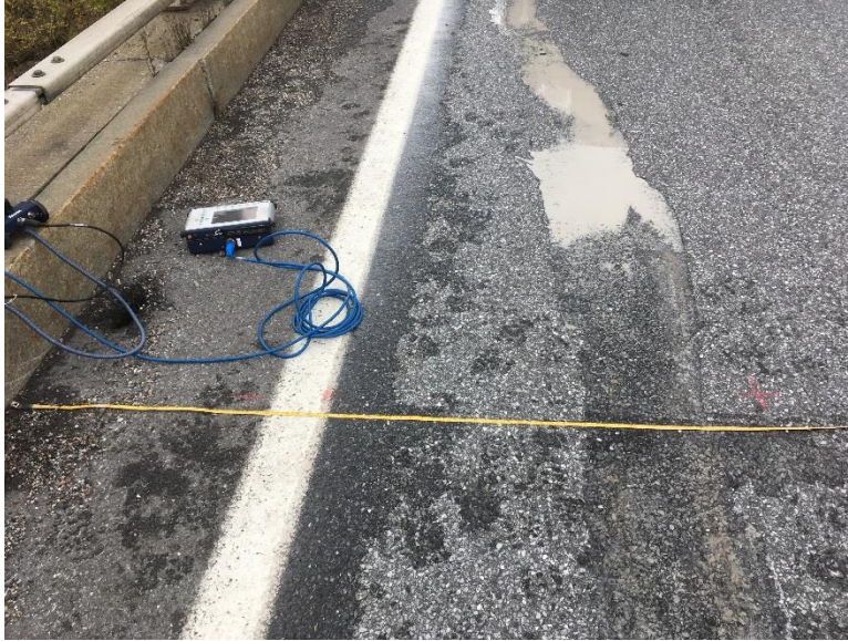
Figure 14: Area 2 GPR Scanning Layout.
