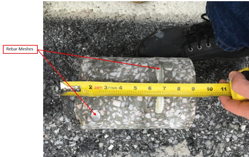
Figure 18: Area 2, L2 Core on Bridge 77. Rebar Meshes were Present.
