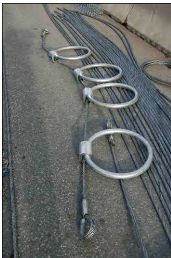
Figure 9 Close-up of Breaking Element.
