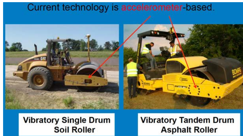
Figure 3. Accelerometers mounted on the rollers (Source: Naras et al., 2015)
