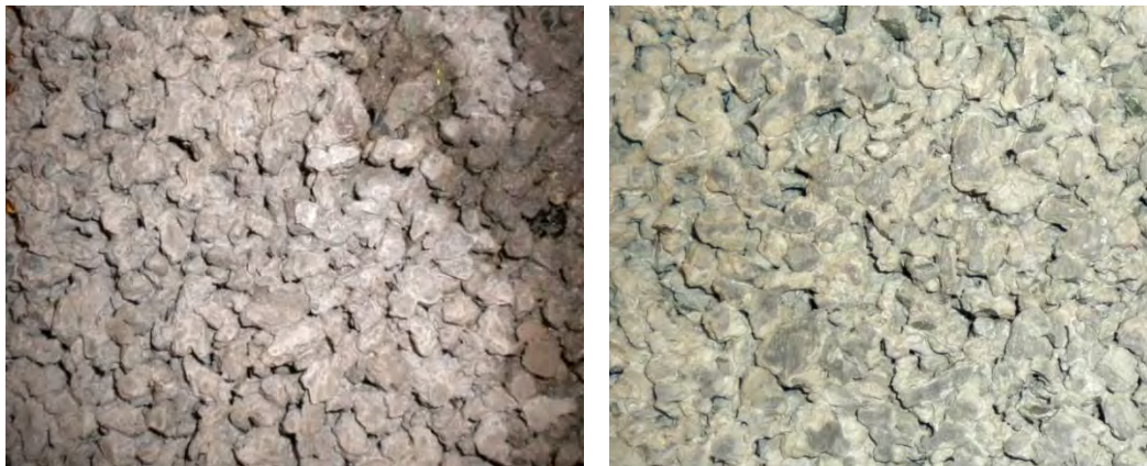
Figure 5.6: Comparison of Porous Concrete Surface after 6 Cycles of Plow Testing: Virgin Sample (left) after 6 Cycles (right)
