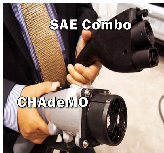
Figure 2 - SAE Combo and CHAdeMO DCFC plug socket designs
