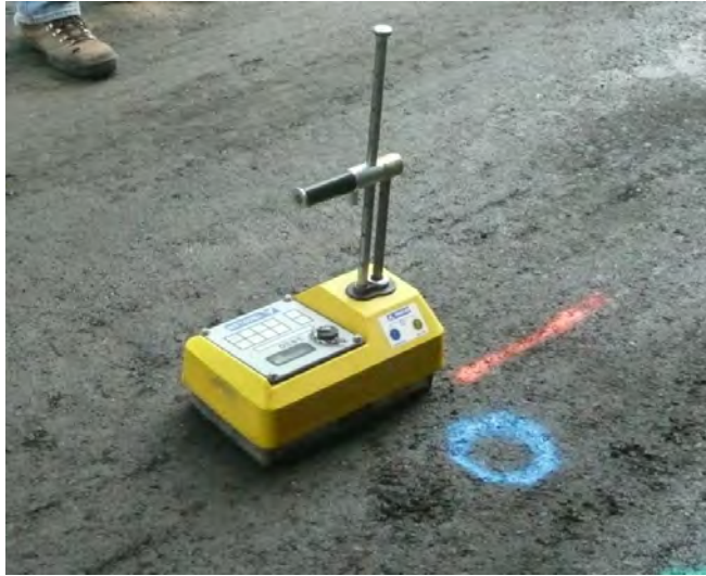
Figure 1 Nuclear Density Gauge (NDG) being used to collect data on a project.
