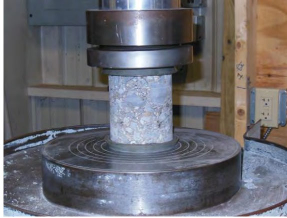
Figure 7 Compression test on a core.
