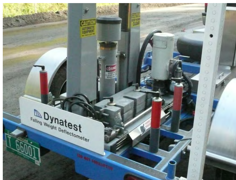
Figure 5 Falling Weight Deflectometer (FWD) being used to collect data on a project.
