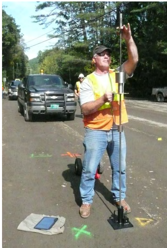
Figure 2 Dynamic Cone Penetrometer (DCP) being used to collect data on a project.
