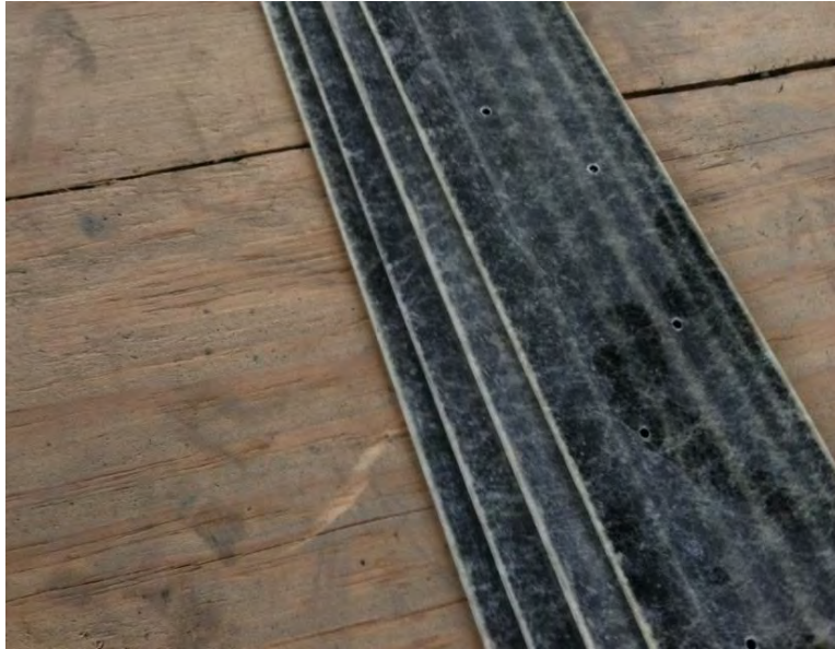
Figure 5 FRP Strips to be installed (VTrans 2014)
