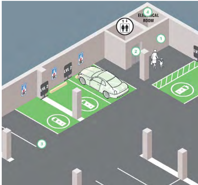
Figure 7.6: Parking Garage Installation
