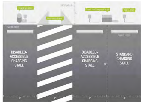
Figure 7.7: Accessible EVCE Design
