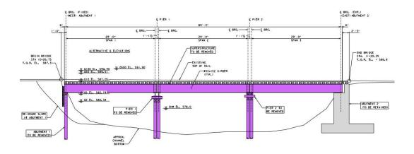
Alternative 6 (Removal of the existing superstructure, piers, and abutment 1) produced similar results as Alternative 5, as removing abutment 1 does not significantly increase the waterway. If the bridge is not put back in service, this alternative is recommended as it removes the piers from the channel and removes abutment 1 now rather than in a future project when the abutment begins to deteriorate over time.
