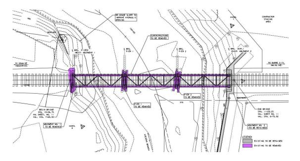
Bridge Alternative 6: Remove Superstructure, Piers, and Abutment 1 (CONT'D)
