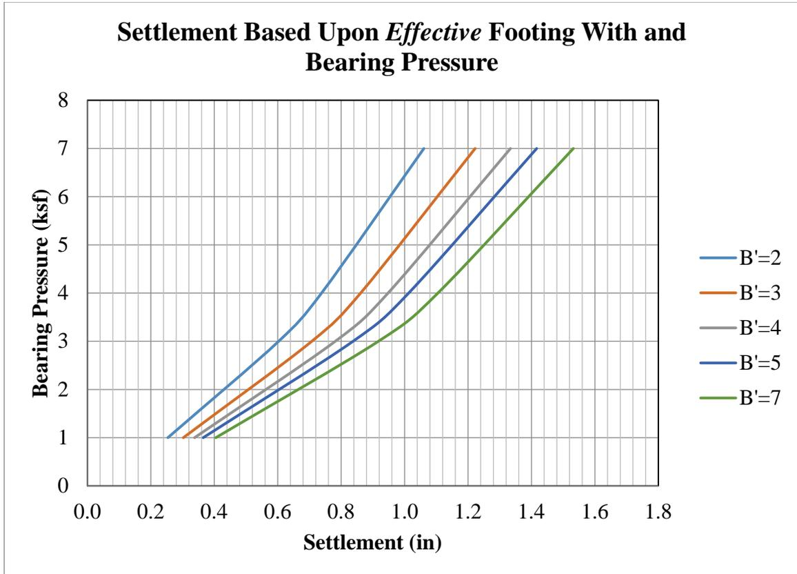
**Figure 4.2:** Settlement vs. Nominal Bearing Pressure (Culvert Wingwalls @ Station 292+21.53)
