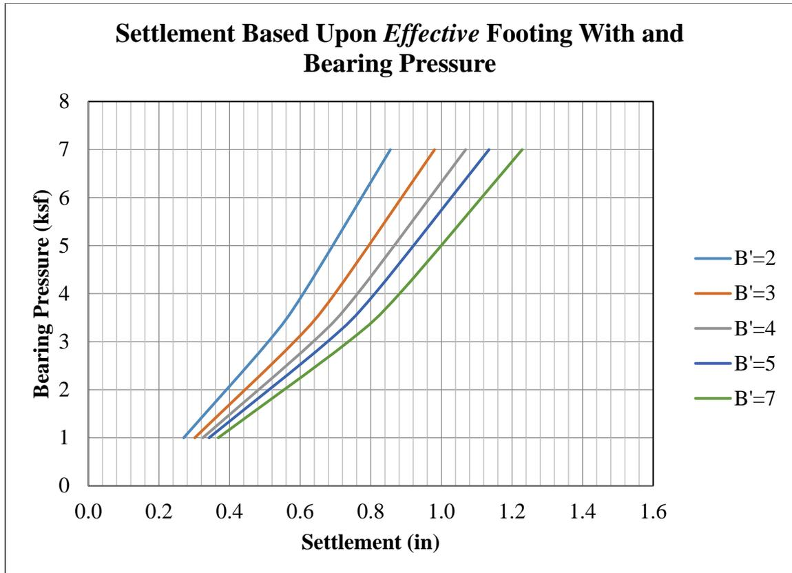
**Figure 4.4:** Settlement vs. Nominal Bearing Pressure (Culvert Wingwalls @ Station 296+33.35)
