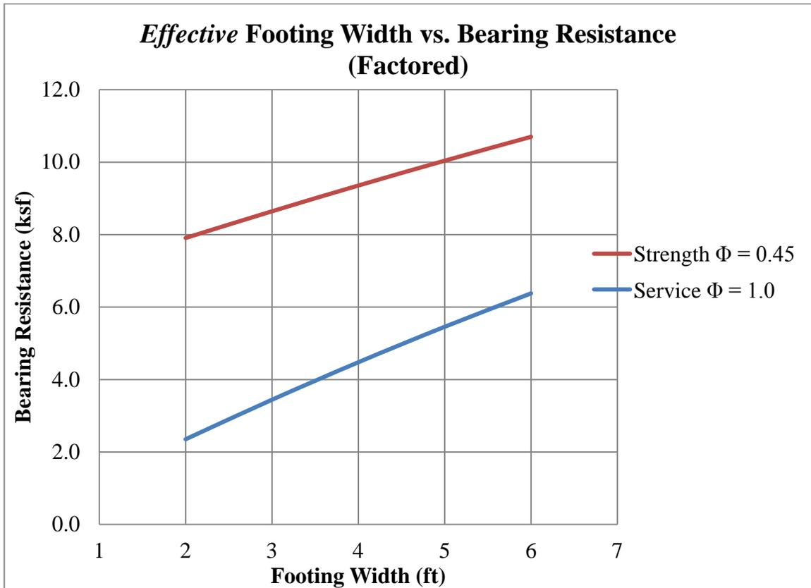
**Figure 4.1:** *Effective Footing Width vs. Bearing Resistance for Culvert Wingwalls @ Station 292+21.53*
