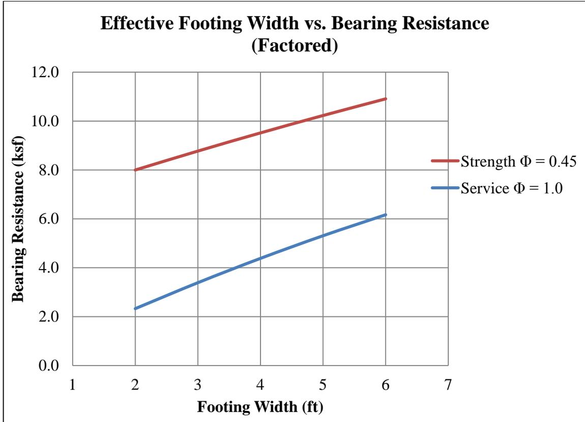
**Figure 4.3:** *Effective Footing Width vs. Bearing Resistance for Culvert Wingwalls @ Station 296+33.35*
