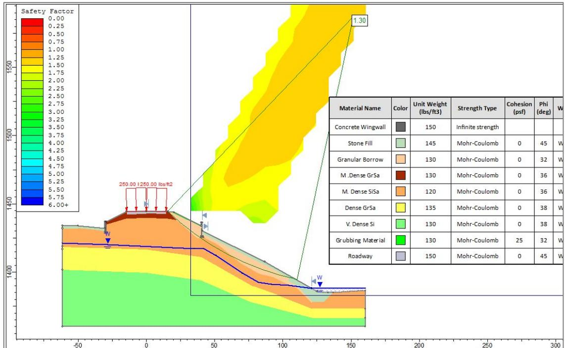
Figure 2.2. Proposed Cross-Section @ Sta 296+33.35
