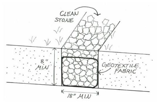
Figure 18: Infiltration Trench
