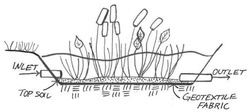
Figure 17: Constructed wetland
