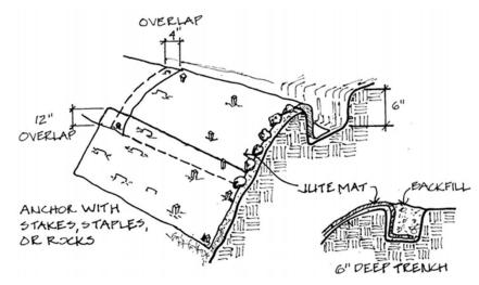
Figure 38: Jute Matting Installation
