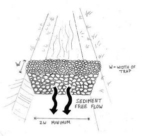
Figure 5: Sediment Trap
