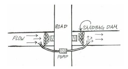
Figure 22: Culvert Installation
