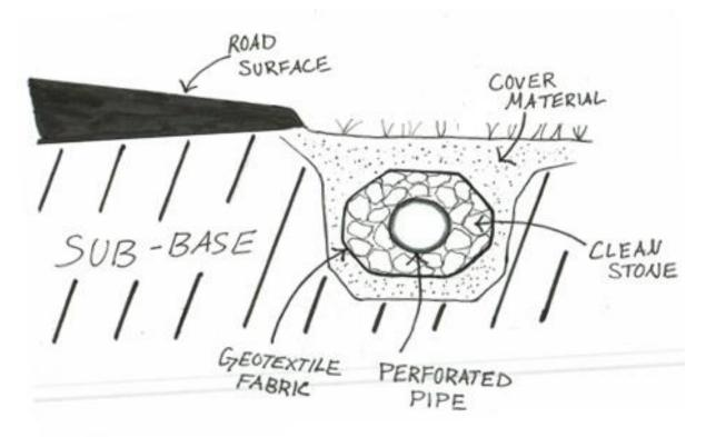
Figure 20: Underdrain
