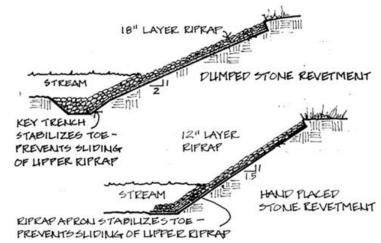
Figure 45: Riprap Revetment System
