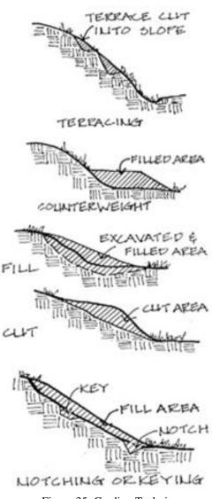
Figure 35: Grading Techniques
