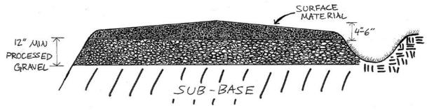
Figure 9: Properly shaped road surface
