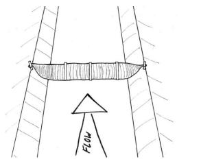
Figure 3: Fiber Roll Section View
