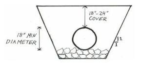
Figure 26: Culvert Installation
