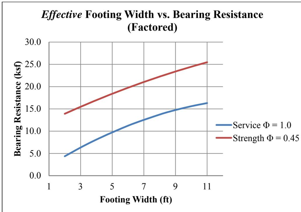
**Figure 4.1:** *Effective Footing Width vs. Bearing Resistance for Culvert Wingwalls*
