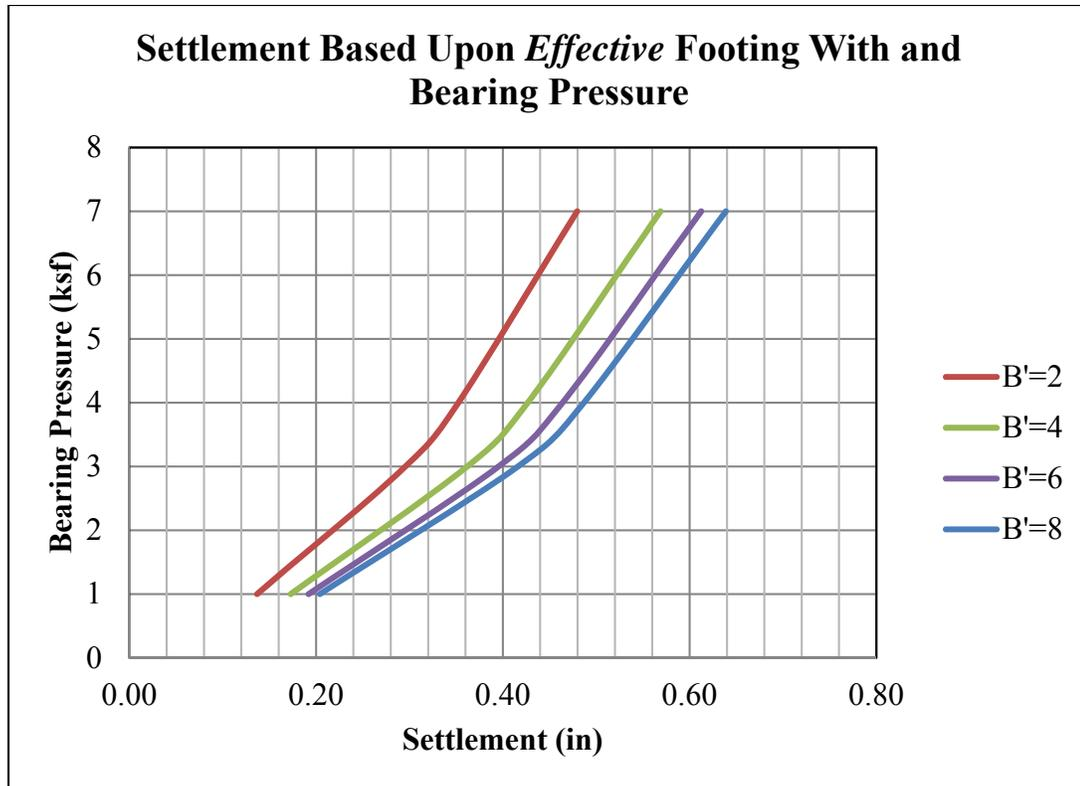
Figure 4.2: Settlement vs. Nominal Bearing Pressure (Wingwalls)
