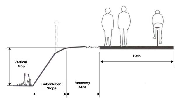
Figure 1: Description of Geometric Parameters Required for Barrier Usage Guideline Adapted from: Vermont Pedestrian and Bicycle Facility Planning and Design Manual. December 2002.
