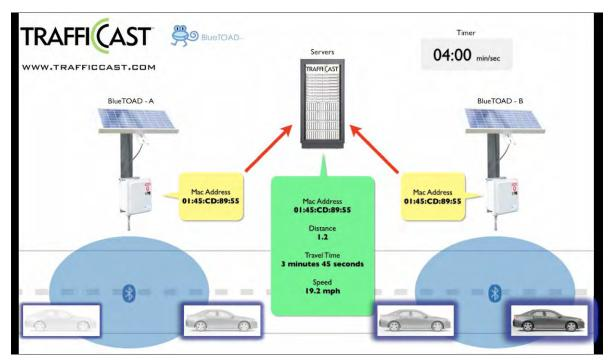
As mobile devices inside vehicles move through the 50 meter detection radius, BlueTOAD identifies and time stamps their Bluetooth MAC Address. Timestamps of subsequent detections determine travel time across the known distance between BlueTOAD units.
