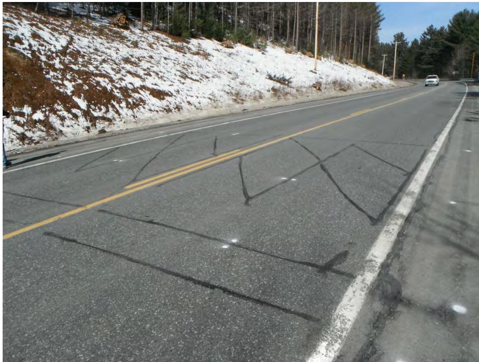
**Figure 2 An example of a Manufactured Cracked Test Site**
