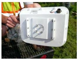
Figure 2: Pole facing side of sensor.
