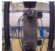
Fig. 1 Pullout test
