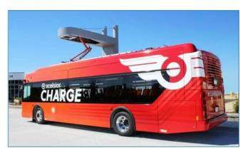
A New Flyer electric bus gets an in-route charge from a pantograph-down overhead conductive charger. This type of charger allows for charging of a bus at a layover or other location away from the depot at speeds faster than most plug in chargers and do not require a maintenance crew member to perform the operation.
