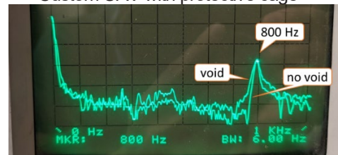
Acoustic spectra of concrete with and without subsurface void
