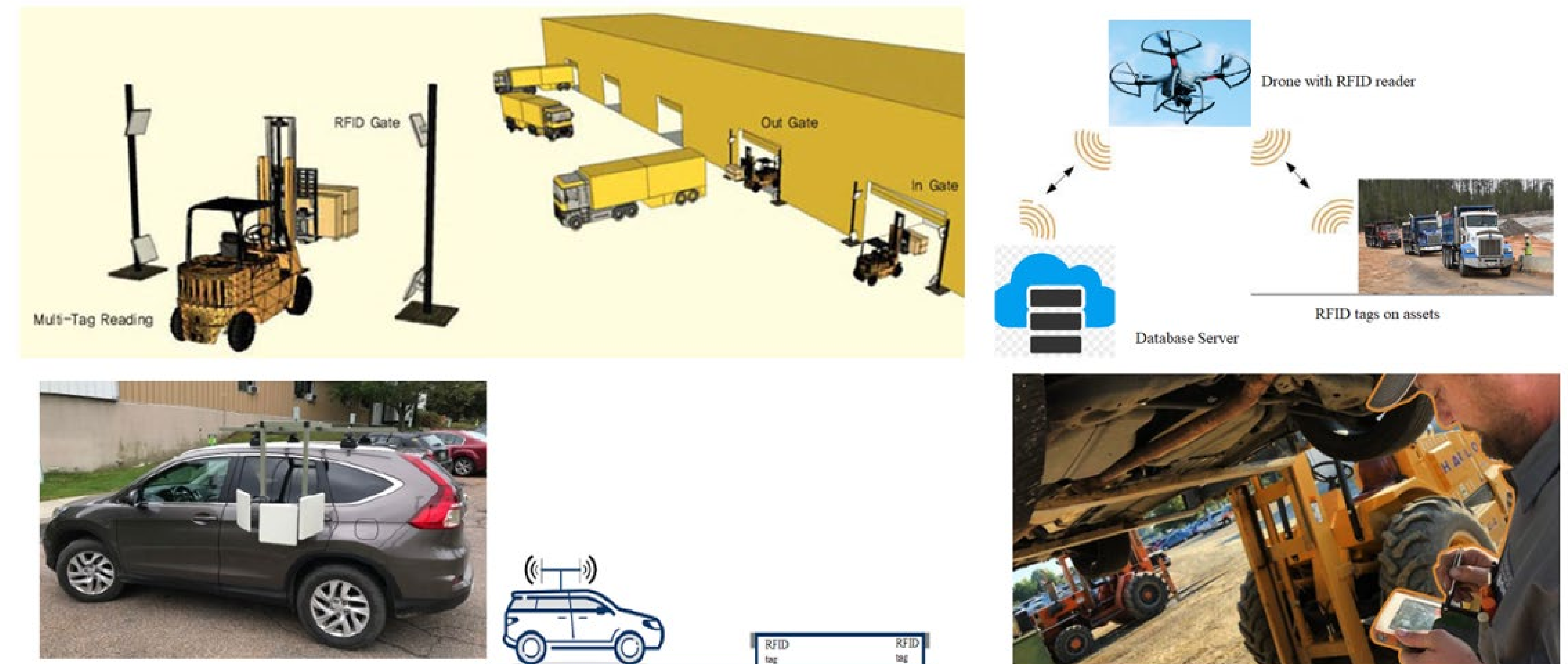
Figure 2. RFID-based transportation maintenance operations and asset management: (upper left) fixed readers in a warehouse (source: [4]); (upper right) a drone-mounted reader in a field; (lower left) a car-mounted reader on the road (source: [4]); (lower right) a handheld reader in a lot.
