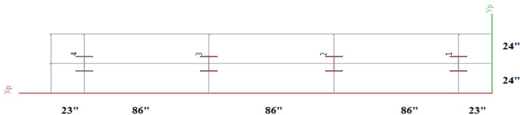
Figure 2.1: Abutment Pile Layout
