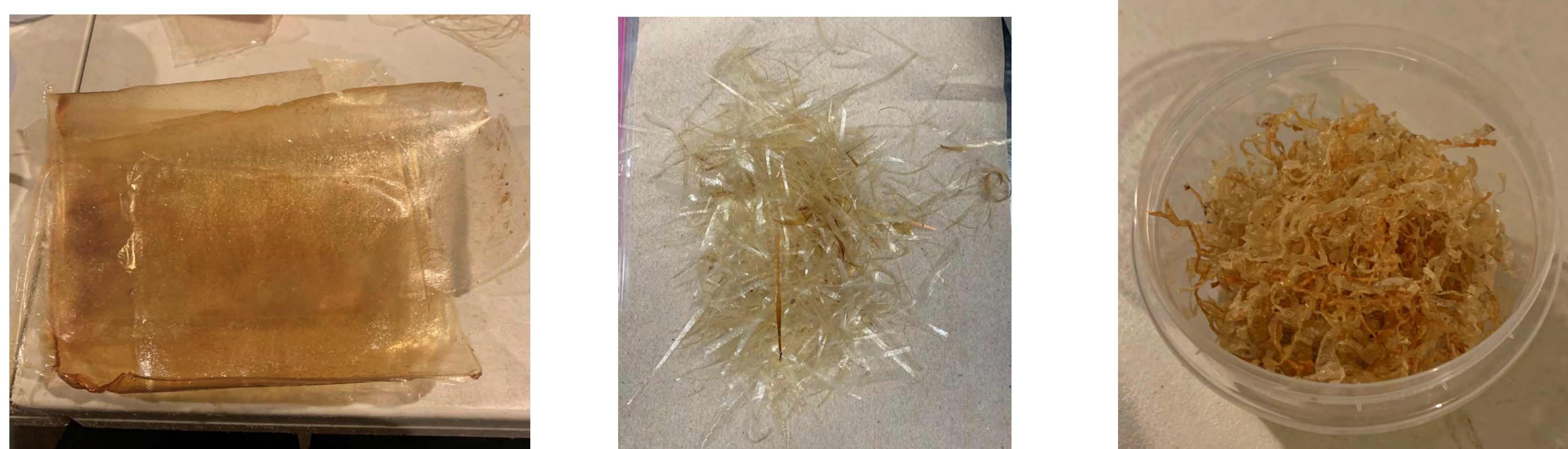
Figure 1. Sheets of shrinking chitosan fibers (left), cut active fibers (middle), pre-shrunk passive fibers (right)
