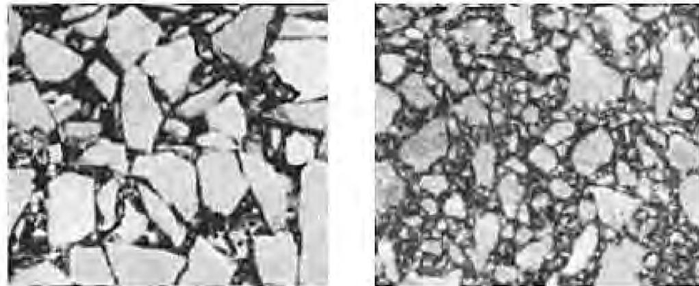
Figure 1. SMA compared to Dense Graded HMA
