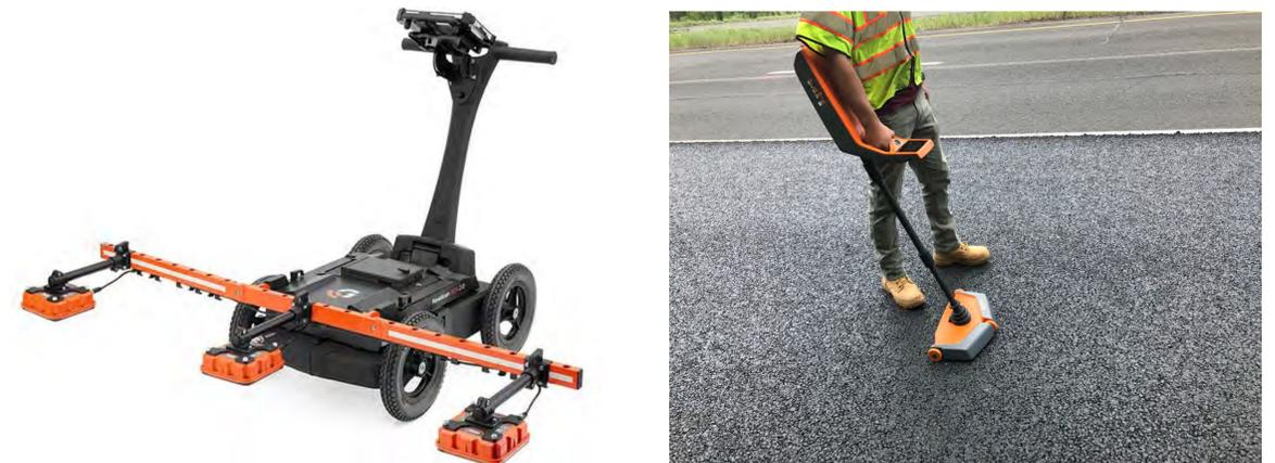
Figure 3. PaveScan GPR Density tool, and MIT-scan pavement thickness tool
