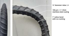
1/2" diameter rebar (#4) 100 µm (.04") thick
