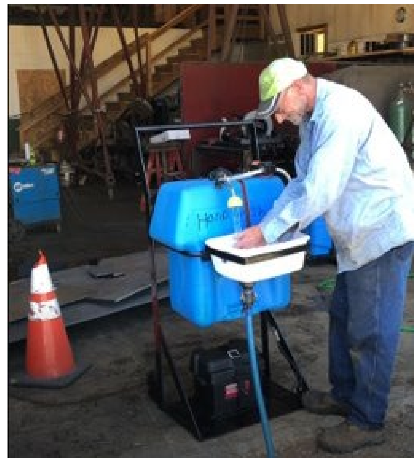
Figure 2: Mobile handwashing station fabricated by Ricky Hayes, District 1
