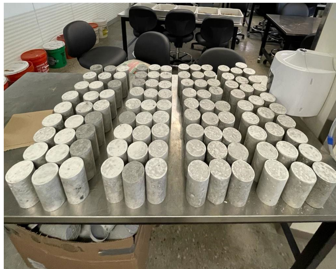
Figure 1. Concrete cylinders right after the demolding process.
