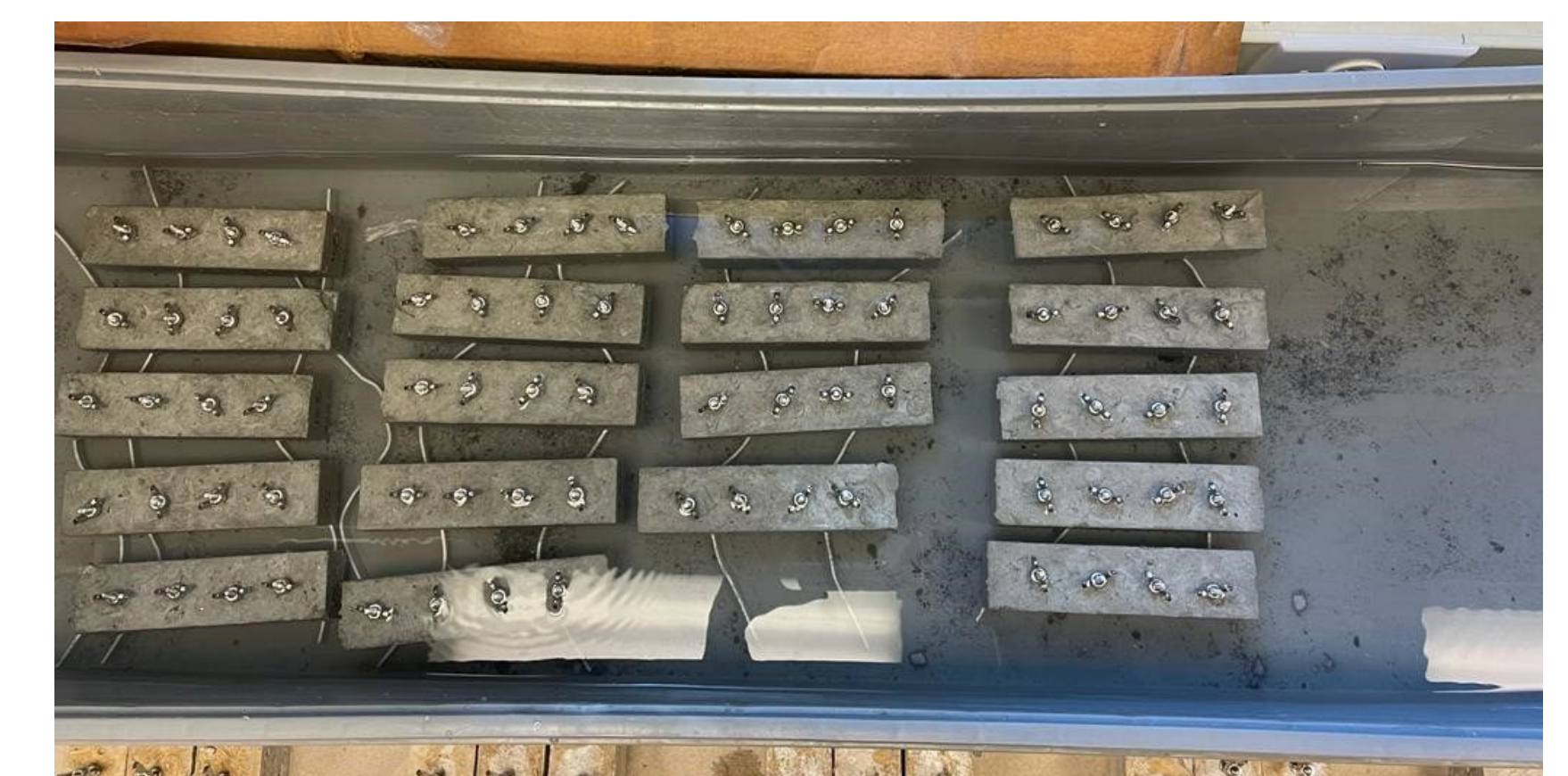
Figure 3. Concrete specimen being tested for compressive strength (Left), Concrete specimens undergoing chloride soaking (Right)
