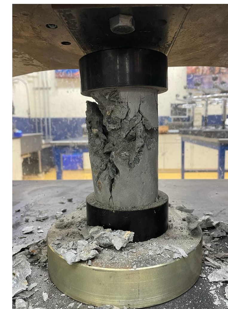
Figure 3. Concrete specimen being tested for compressive strength (Left), Concrete specimens undergoing chloride soaking (Right)
