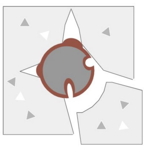
Rebar corrosion often determine the lifetime of concrete infrastructure, and limits the average bridge deck life to only 30-40 years. [1]
