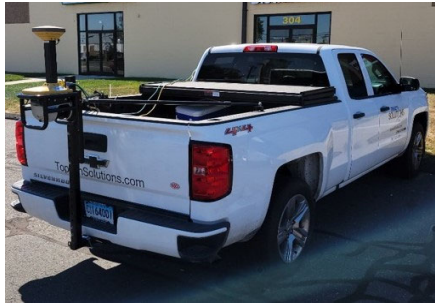
Figure (Left): Realistic Dimensioning – Mapping One (RD-M1) surface scanner mounted on truck
