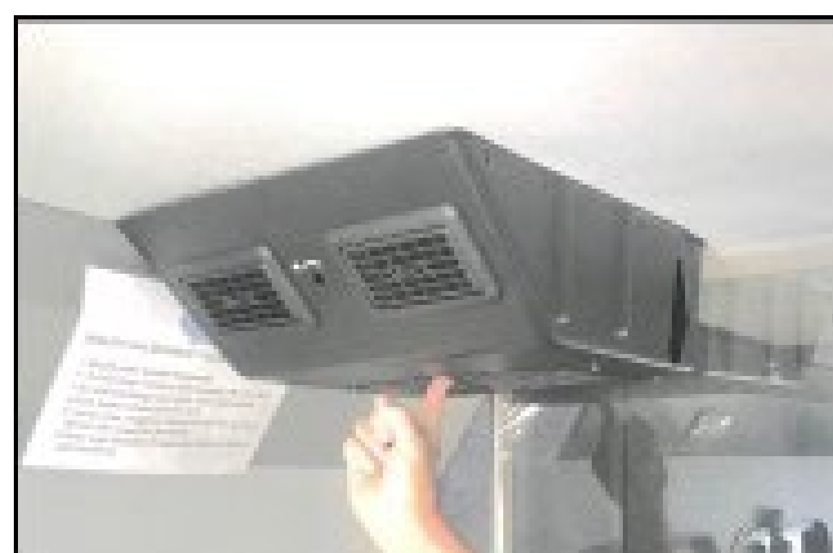
Figure 2. Enclosed Pro Air HEPA 3 filtration unit and “Glove Box” experimental paradigm
