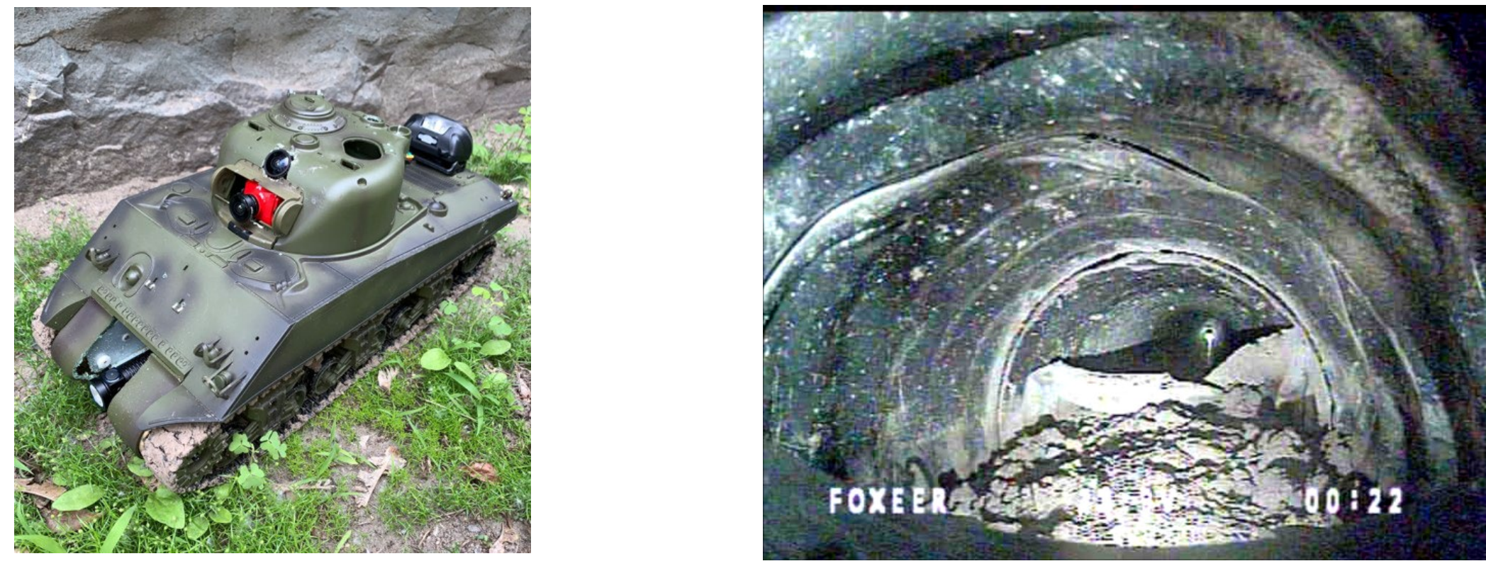
Figure 1. Left: HIVE tank. Right: Culvert with sediment buildup.
