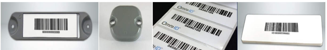
Fig. 7: RFID tags used in the experiment. (From left to right is tag 1 (Omni-ID Flex 800), tag 2 (Omni-ID Exo 750), tag 3 (Omni-ID IQ 800), and tag 4 (Omni-ID Flex 1200).).
