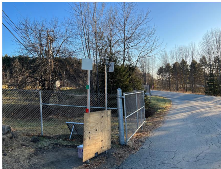
(b) RFID reader packaged in a waterproof box
