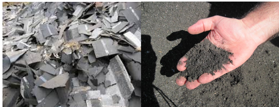
Left: As produced architectural waste shingles; Right: resized processed waste shingles [image sources: Wisconsin Dept of Natural Resources and North Carolina Department of Environment Quality]
